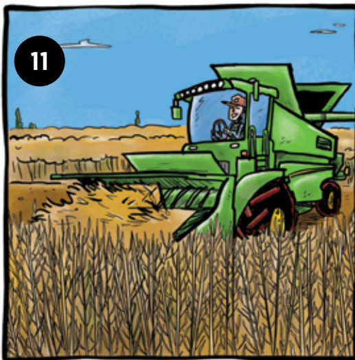
Seed colour determines maturity and indicates when the canola crop is ready for harvest. A combine is used to get the dry canola seeds out of the golden yellow pods.
