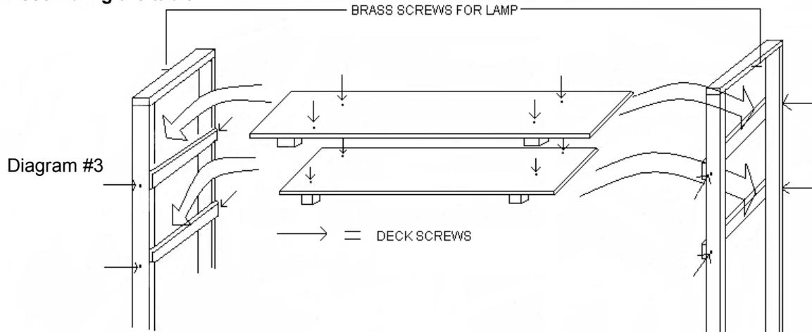
1. It is useful at this point to have either a small swarm of children for assistance or four hands. Also make sure that the shelves (which should be about 24" wide) easily fit between the upright 2x4s of the end pieces (which should be 24" apart). If not, trim a bit to fit.
