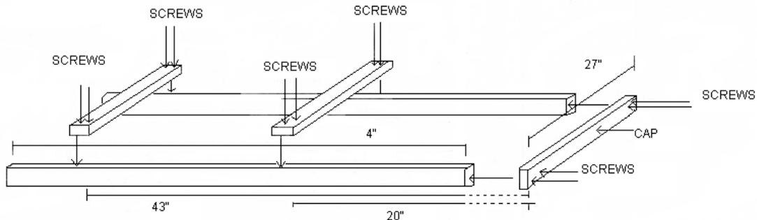
1. Lay two 4" 2x4s on their narrow side on the floor parallel to each other and 24" apart (see diagram #1).
